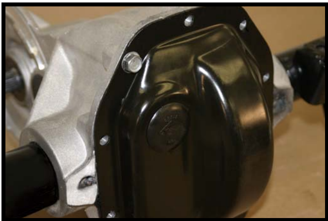
Fig. A-3 Differential Cover Plate, Assembled
