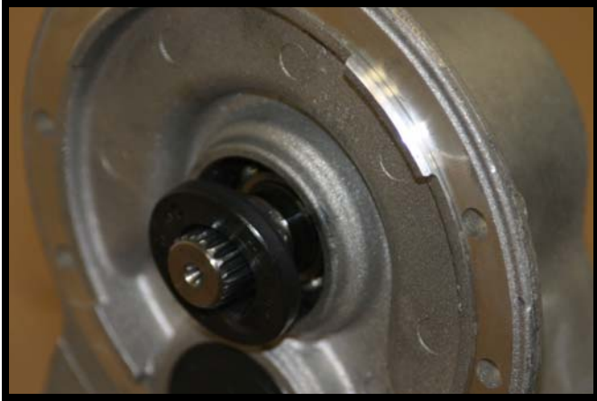
Fig. A-11 Removing Oil Seal from Input Gear Assembly
