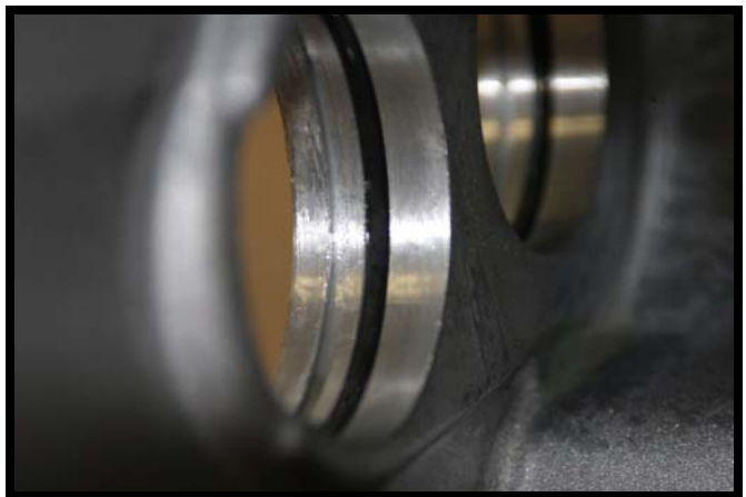
Fig. A-21 O-Rings Removed from Axle Housing
