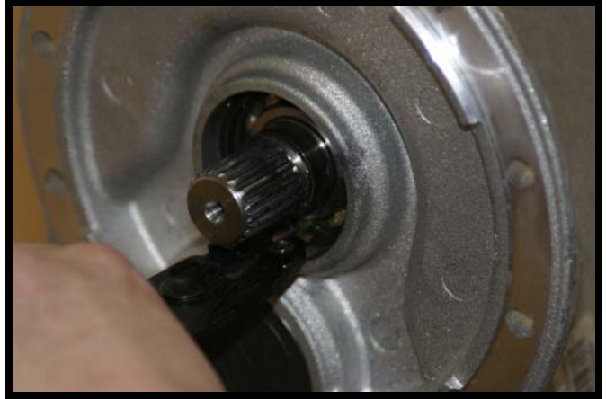
Fig. A-11 Installing Retaining Ring into Input Gear Assembly and Axle Housing
