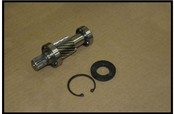
Fig. A-13 Oil Seal, Retaining Ring, and Input Gear (With Two Bearings Attached) Removed
