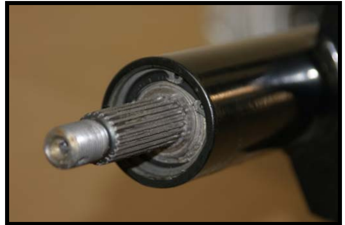
Fig. A-9 Axle Shaft, Outer Snap Ring, and Bearing Shown Assembled in Axle Tube
