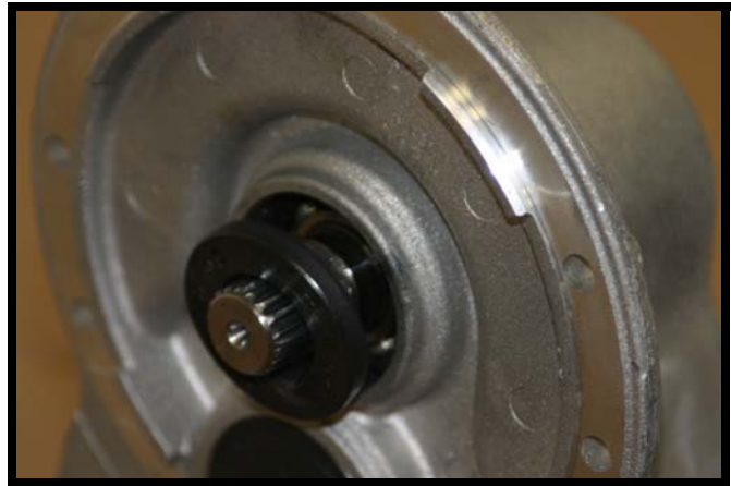
Fig. A-12 Installing Oil Seal into Input Gear Assembly
