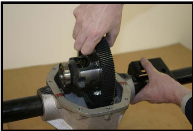
Fig. A-16 Removing Differential-Carrier Assembly from Axle Housing
