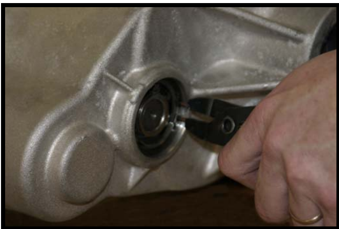
Fig. A-19 Removing Retaining Rings
