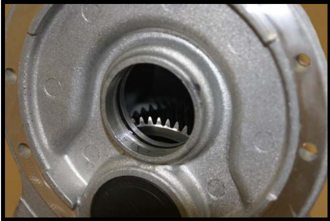
Fig. A-9 O-Ring Installed in Input Gear Assembly
