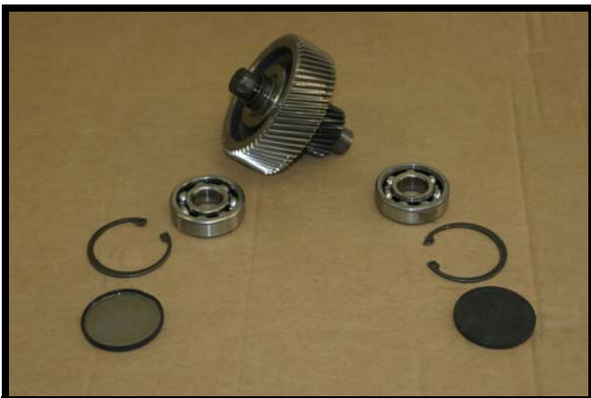
Fig. A-2 Intermediate Gear Assembly Components
