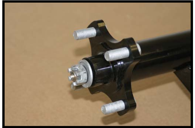
Fig. A-14 Assembled End of Axle Tube
