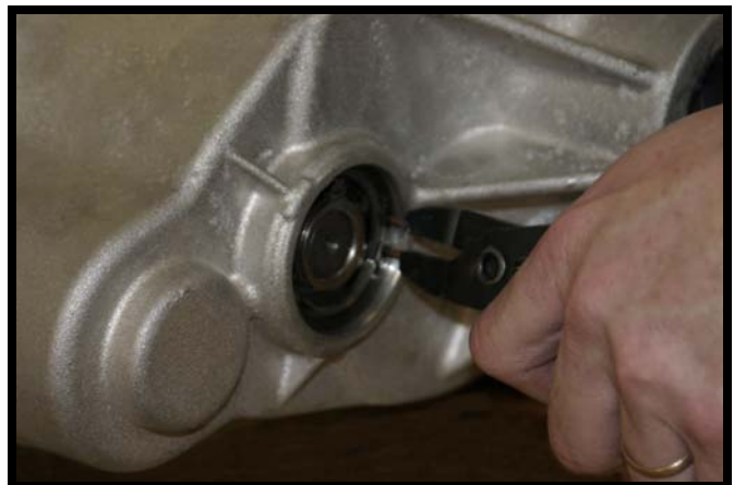
Fig. A-4 Retaining Rings Installed
