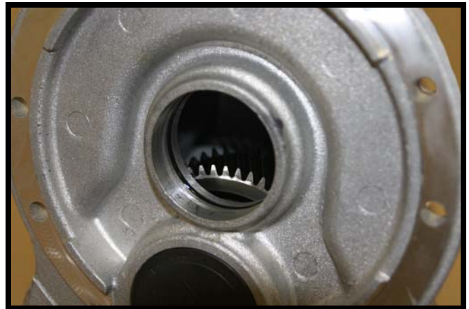
Fig. A-14 Axle Housing with Input Gear Assembly and Hardware Removed
