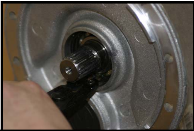
Fig. A-12 Removing Retaining Ring from Input Gear Assembly
