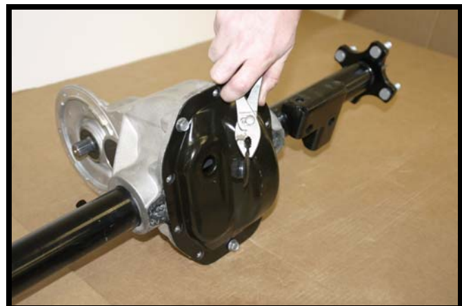
Fig. A-2 Rubber Plug Removal, Step 2
