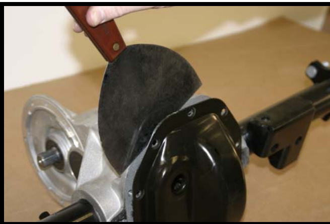
Fig. A-5 Removing Differential Cover Plate
