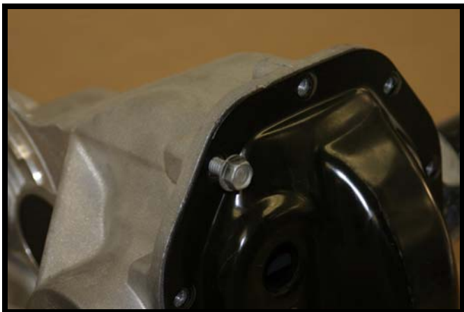
Fig. A-4 Removing Bolts from Differential Cover Plate
