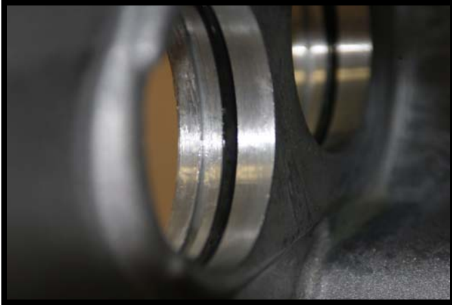
Fig. A-1 Intermediate Gear Assembly O-Rings Installed
