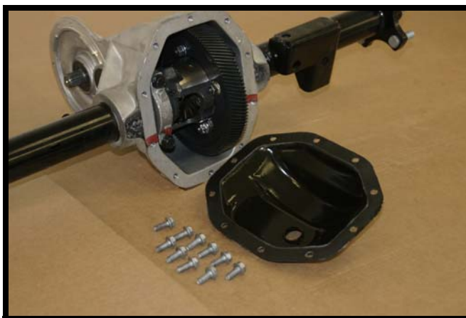
Fig. A-6 Bolts and Differential Cover Plate Removed
