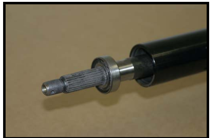
Fig. A-10 Removing Axle Shaft From Axle Tube
