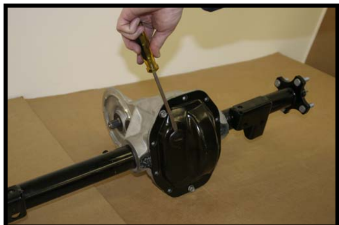
Fig. A-1 Rubber Plug Removal, Step 1
