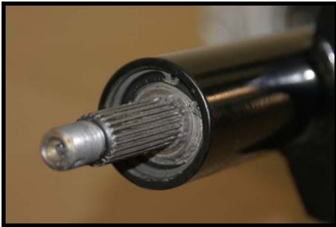
Fig. A-13 Axle Shaft, Outer Snap Ring, and Bearing Shown Assembled in Axle Tube
