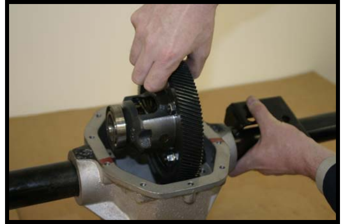
Fig. A-7 Installing Differential-Carrier into Axle Housing
