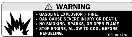
GASOLINE WARNING DECAL (ON VEHICLE FRAME NEAR FUEL TANK)
