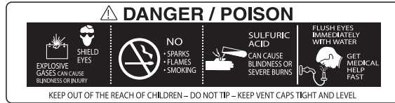
BATTERY DANGER DECAL (ON BATTERY CAPS OR ON BODY UNDER SEAT)
