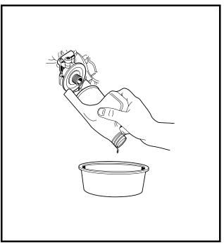
Figure 20 Remove Engine Oil Filter
