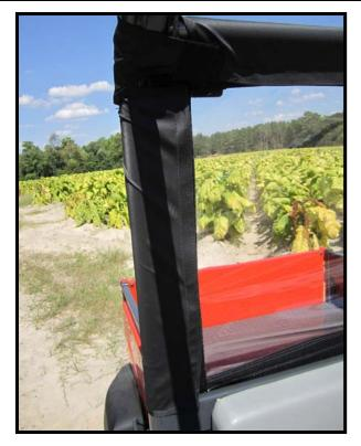
3. Attach rest of the velcro around the roll cage
