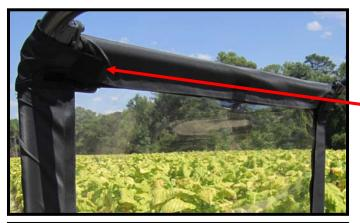
1. Wrap the velcro around the rear top bar on the roll cage. Ensure that the end flaps are secured around the bar as shown in the pictures.
