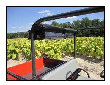
A - The dust panel can be rolled up by undoing step 3, rolling the window up from the bottom, and securing with the three straps at the top of the window as shown.
