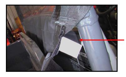
4. Peel off adhesive backing on the bottom velcro piece and attach to the back of the square horizontal bar behind the seat.
