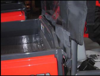
2. Allow the bottom end of the back panel to drape behind the dump bed.
