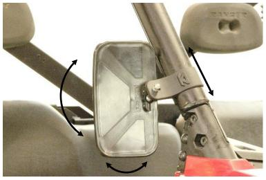
Adjust the mirror up and down the roll cage and angle as needed. Fully tighten locknut.
