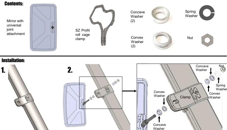
Open the clamp with two hands and snap around roll cage. Be careful when releasing the clamp to avoid pinching fingers. The SZ logo should face forwards.
