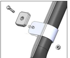
Adjust windshield as needed and tighten bolts.
