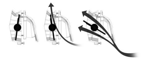
The vent has 3 positions: Closed, Defog, and open.
