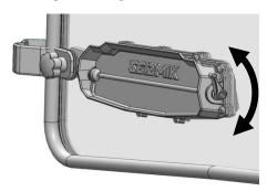
Turn handle to adjust vent. If the vent seems too tight or too loose, it can be adjusted by turning the T10 Torx screw in the handle.
